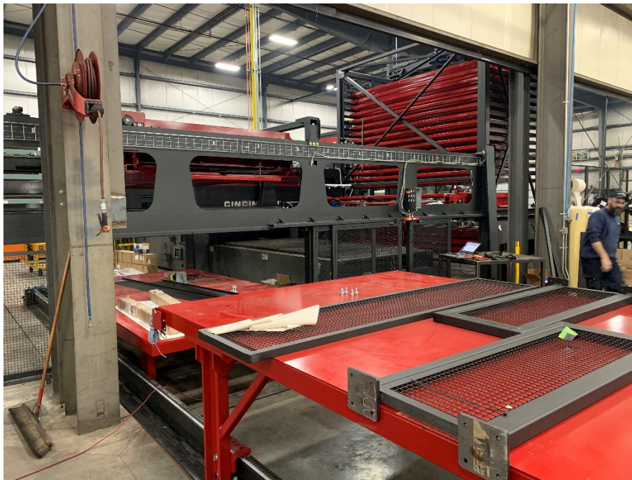
Mega Fab Robotic Material Handling system unload area with sheet tower and laser in the background.
